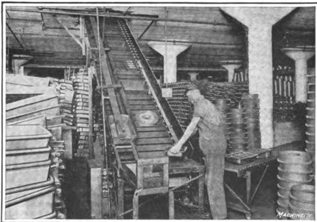
Fig. 35—An elevator raises the work to the upper floor in the Willys-Overland Co.'s plant. This equipment, installed by the Link-Belt Co., Chicago, Ill., consists of an apron-type conveyor with cleats to prevent the work from slipping back. A chute at the left returns the tote boxes to the lower floor
